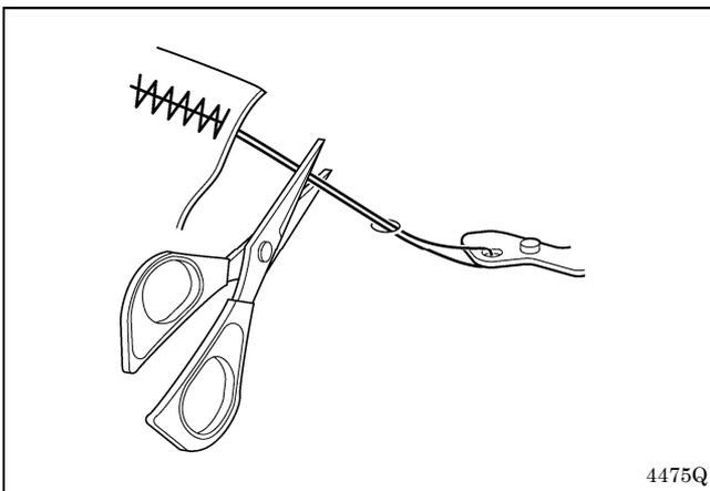
2. If the upper thread trailing length is 40 mm or more, or if the upper thread tension is weak and the upper thread does not form a good seam at the first stitch, the end of the thread that is being held by the thread nipper may become wound around the seam. Furthermore, if using thick thread that is #30 or higher or if the thread trailing length is too long, an error "E692" may occur. In any of these cases, use scissors to cut the thread without pulling it up too hard.
