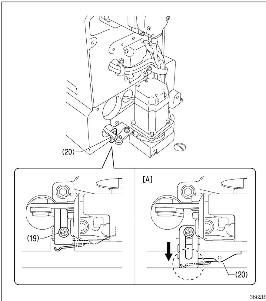
1. Loosen the screw (19), and then install the machine head switch (20) in the position shown in the illustration.
