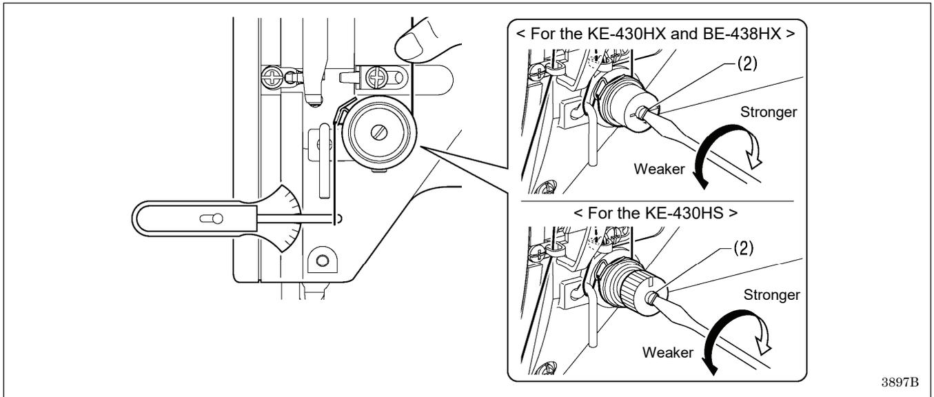
Adjust by turning the shaft (2) with a screwdriver.
