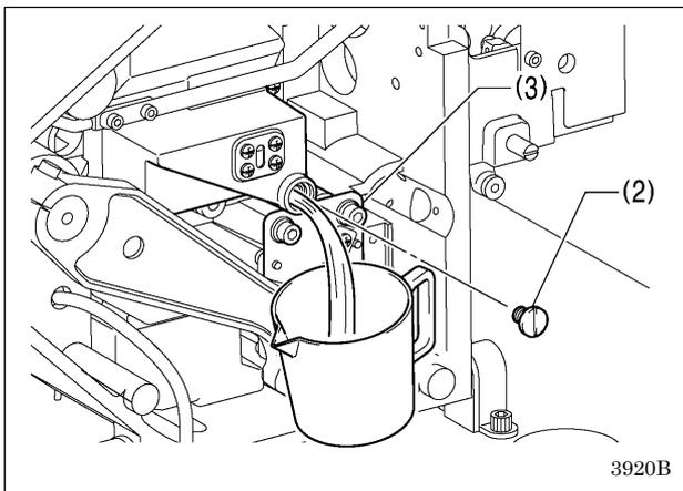
4. Have an oil pan ready, and then remove the screw (2).
