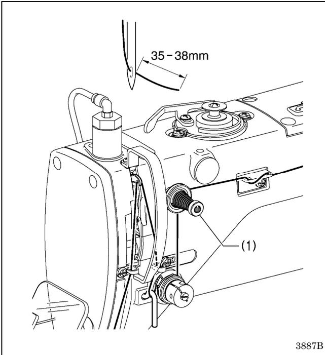
1. When using the thread nipper device, turn the tension nut (1) (sub-tension) to adjust the upper thread trailing length to 35 - 38 mm.
