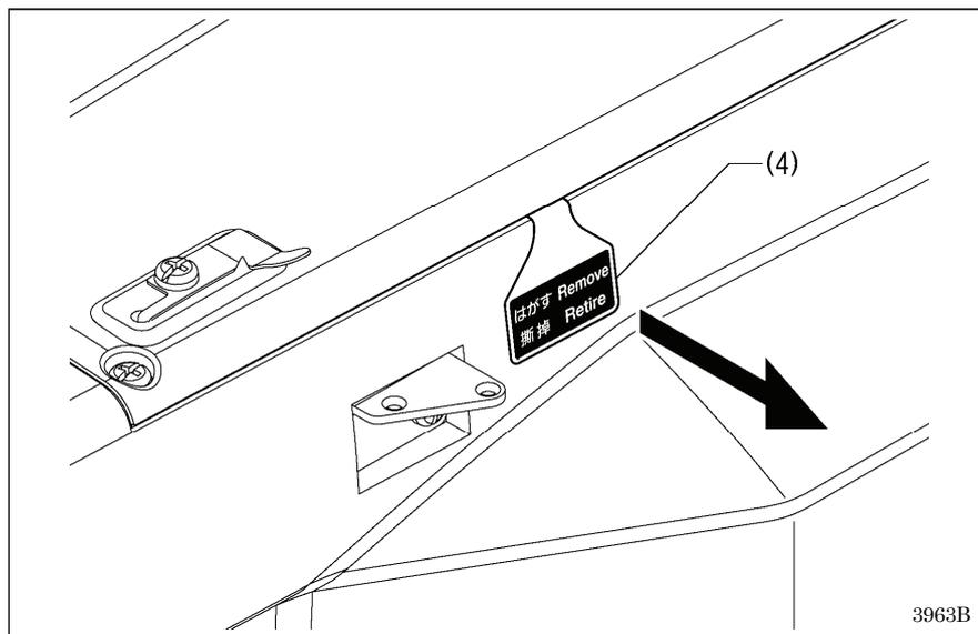
Pull the seal (4) in the direction of the arrow to remove it.
