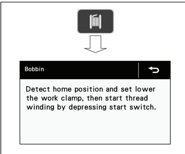
1. First, press the bobbin key
