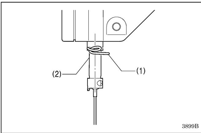
Check that needle bar bush thread guide D (1) is at the middle of the needle bar (2).
