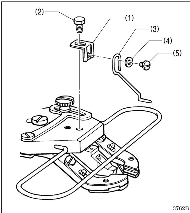
If you would like the button to be raised up more after it is sewn without replacing the button clamp spacer, install the accessory button lifter spring.
