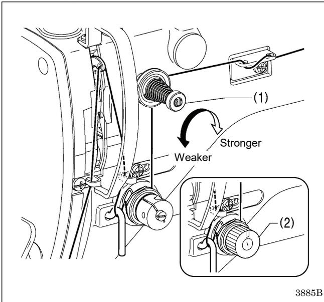
Use the digital tension or the tension nut (2) to adjust the tension as appropriate for the material being sewn. (Refer to "Setting the tension value".)
