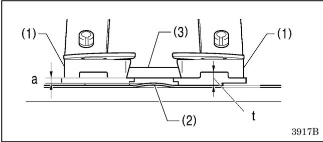
The button lift amount can be adjusted in order to change the clearance (a) between the material (2) and the button (3) by changing the thickness (t) of the button clamp spacer (1).
