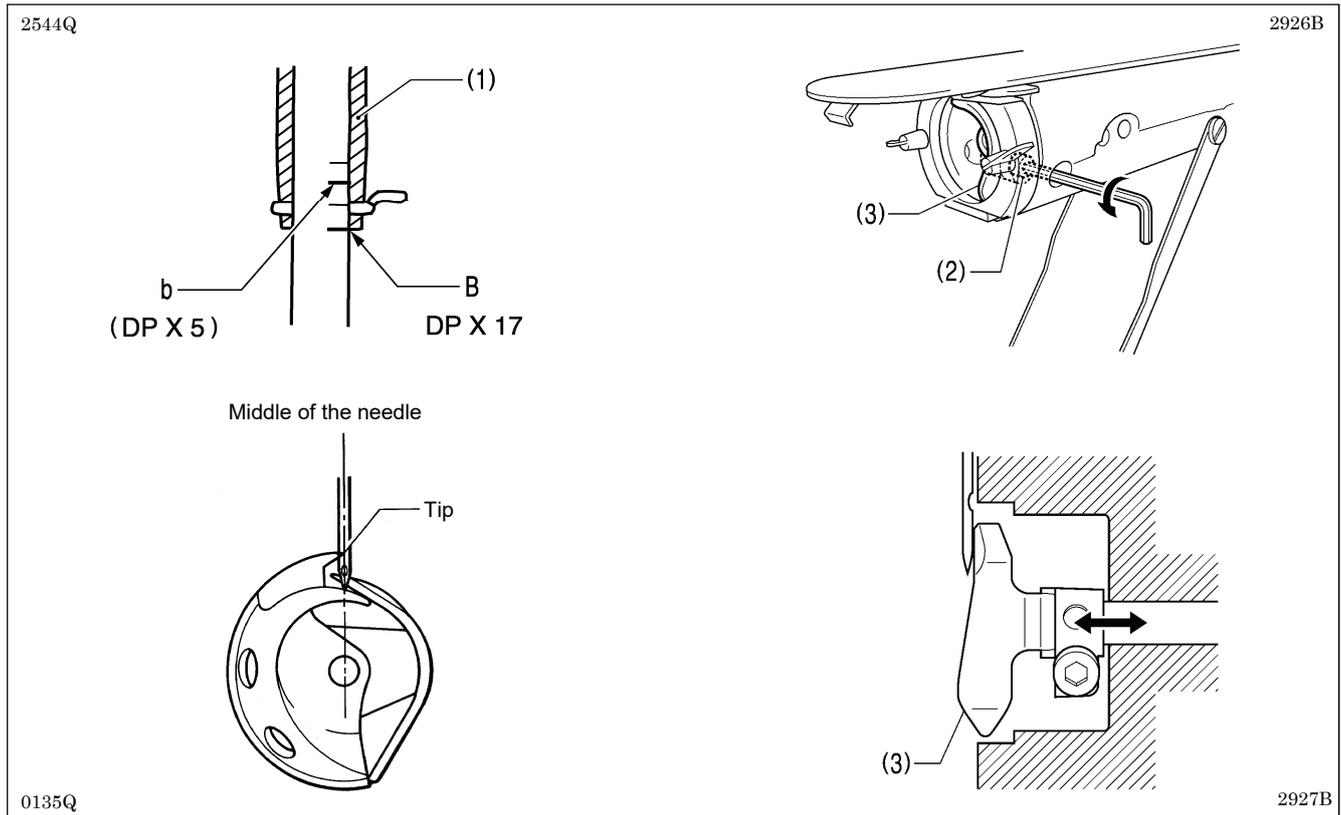
1. Turn the pulley in the direction of the arrow to raise the needle bar from the lowest position until the lowest reference line on the needle bar (reference line B) is aligned with the lower edge of the needle bar bush (1).
