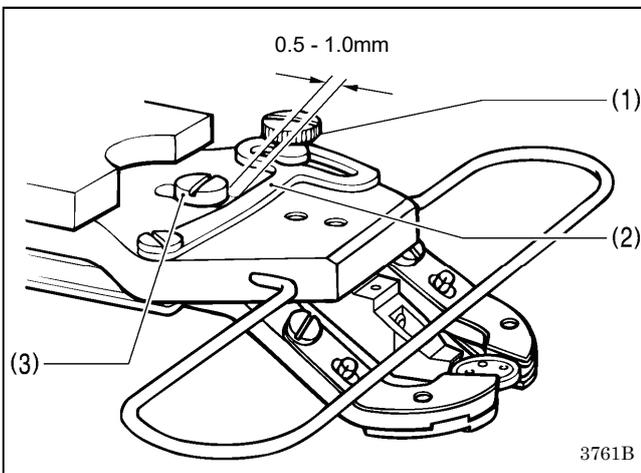
1. Insert a button in the button clamp, and then confirm that the button is securely held by the clamp and that the button can be turned by hand.
