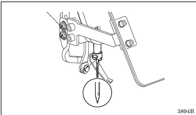
Always check that the tip of the needle is not broken and also the needle is not bent before starting sewing.
