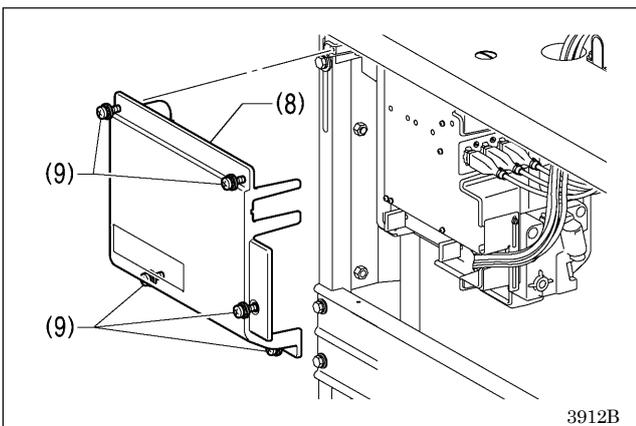
8. Use the five screws (9) to tighten the cover (8) of the control box.
