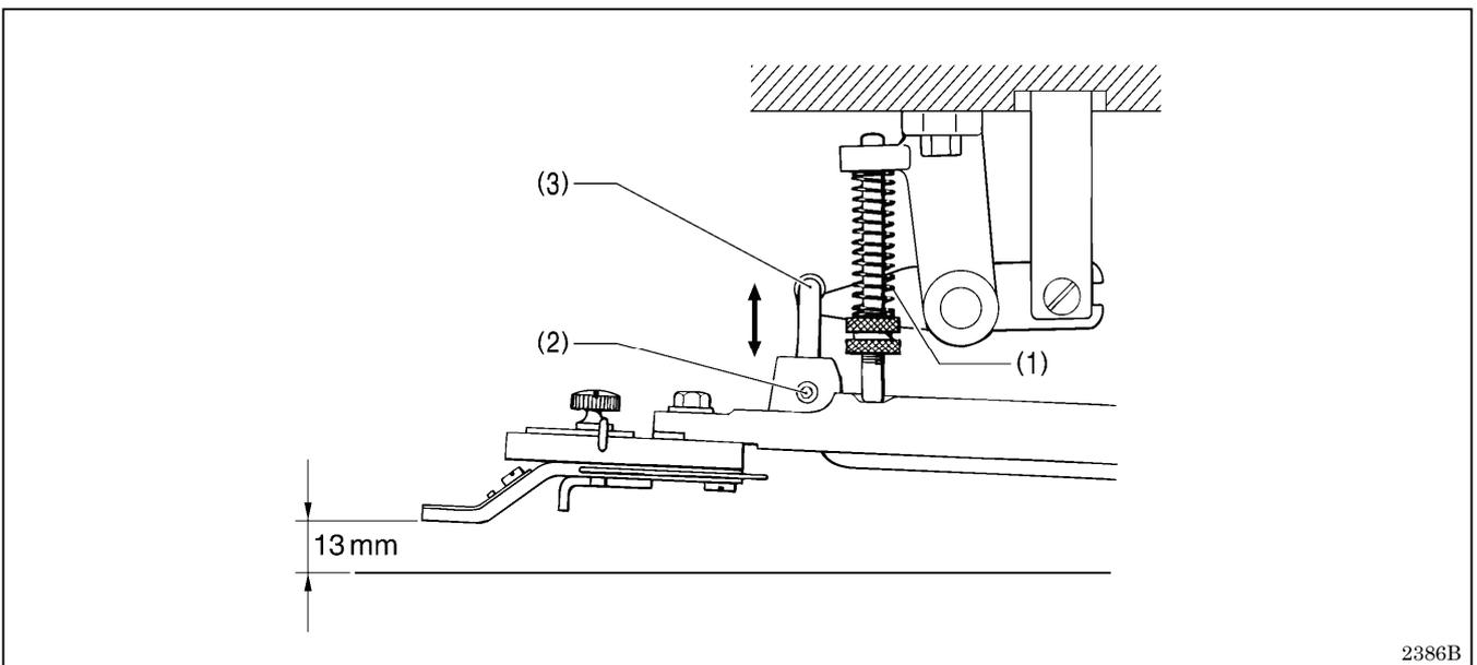
Remove the spring (1), loosen the set screw (2) and adjust the button clamp holder hook (3) by moving it up and down.
