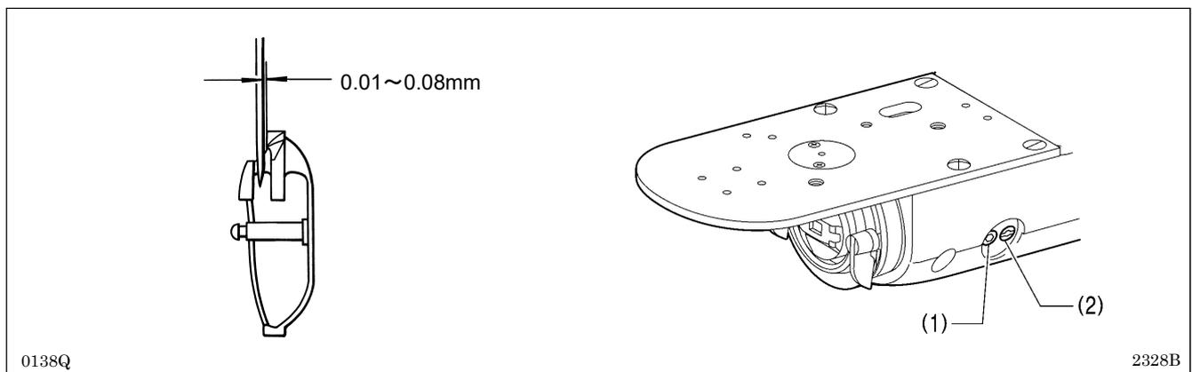
Turn the pulley in the direction of the arrow to align the tip of the shuttle hook with the needle center line. Then loosen the set screw (1) and turn the adjusting stud (2) to adjust so that the clearance between the needle and the tip of the shuttle hook is 0.01 - 0.08 mm.
