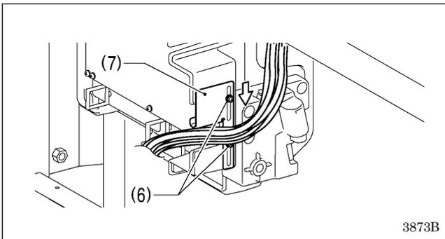
6. Close the cord presser plate (7) in the direction of the white arrow, and secure it by tightening the two screws (6).
