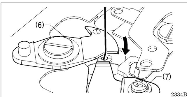
Select an accessory movable knife spacer (11) which allows the movable knife (6) to cross over the fixed knife (7) with a force that is as gentle as possible while still allowing the thread to be trimmed.
