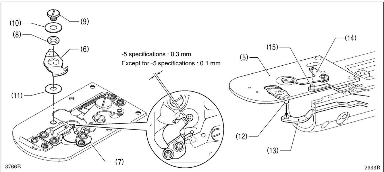
4. Install new fixed knife (7) in the position shown in the illustration.
