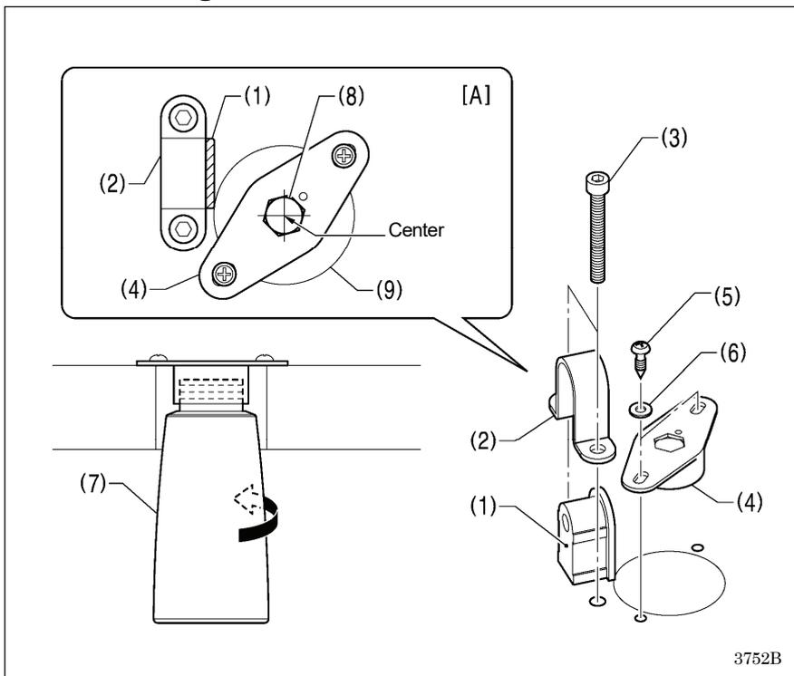
Before installing the oiler, provisionally install the rubber cushion (1) and the hinge holder (2) to the table with the two bolts (3).
