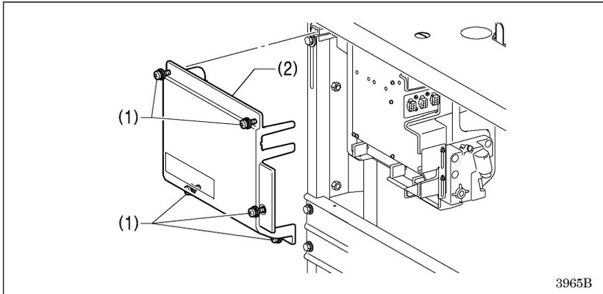
1. Remove the five screws (1), and then remove the control box cover (2).
