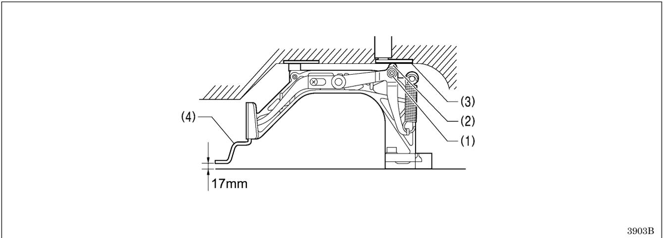
1. Loosen the bolt (1) and move the work clamp arm lever plate (2) up or down to adjust.
