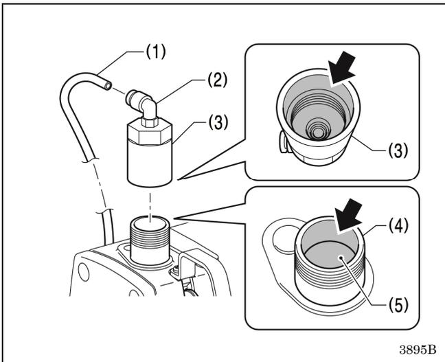
1. Disconnect the tube (1) from the elbow union (2), and then remove the air cylinder cover (3).
