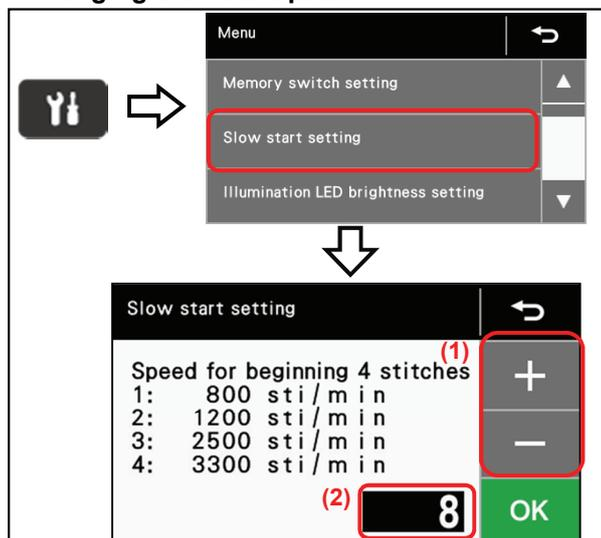
\* This setting cannot be made when the memory switch No. 100 is set to "OFF".
