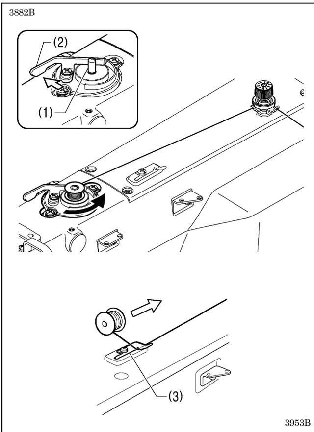
2. Place the bobbin onto the winder shaft (1).
