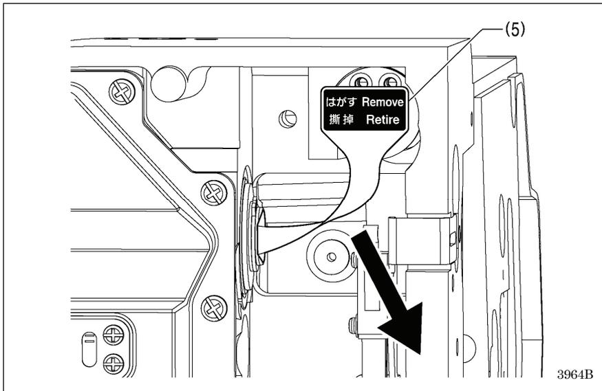
Remove the seal (5) completely.
