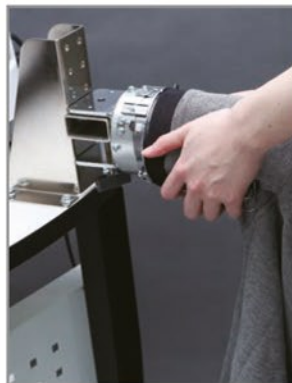
Stretch the piece over the special frame
