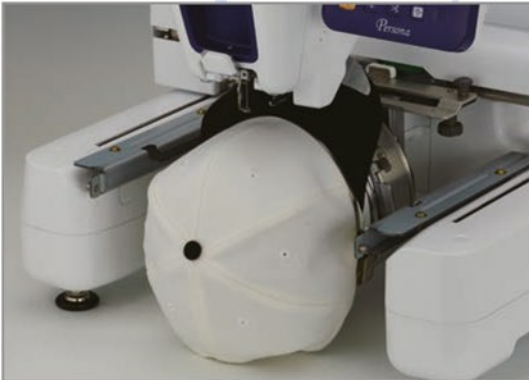
Set completed cap directly onto the machine
