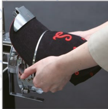
Stretch the cap over the frame
